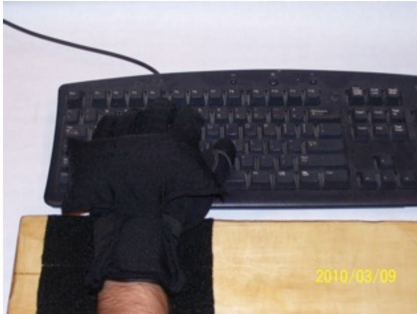
Figure 1. Final Prototype showing the glove and platform attached with a keyboard as a reference.
